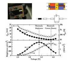
The formation of electric double layers (EDLs) and an emissive p-n junction in light-emitting electrochemical cells are studied. At low applied voltage, EDLs with a thickness of  $\approx 2-3$  nm form at the electrode interfaces, and at voltages exceeding the bandgap potential of the emissive conjugated polymer, a light-emitting p-n junction forms in situ, with a steady-state structure that depends strongly on the applied voltage.
