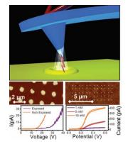
Atomic force microscopy (AFM)-based lithography of SU-8 ultrathin films and its applicability for the fabrication of nanodevices are investigated. It is shown that SU-8 presents outstanding insulating properties and extremely high dielectric strength. A physical-chemical mechanism responsible for the AFM-based patterning is proposed and the potential of this AFM nanopatterning demonstrated by the prototyping and testing of nanoelectrode arrays.
