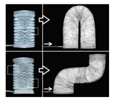
Soft pneumatic actuators based on composites consisting of elastomers with embedded sheet or fiber structures that are flexible but not extensible combine soft lithography, for fabrication, with the principles of origami, for structural design. These actuators respond to pressurization with a wide range of motions, such as bending, extension, contraction, and twisting.
